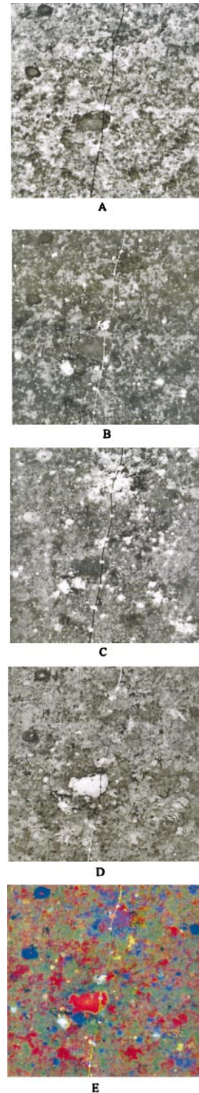
Fig. 1. Grayscale images of the Crosby's Hump site produced by the (A) reflectance (488 nm); (B) green (520 nm) fluorescence; (C) orange (580 nm) fluorescence; and (D) red (685 nm) fluorescence FILLS channels, and (E) a composite pseudocolor RGB presentation of the fluorescence channel data. To make the RGB image, the red fluorescence channel was mapped to the red display channel, the green fluorescence channel to green, and the orange fluorescence channel to blue. The images are each 824 × 824 pixels.
